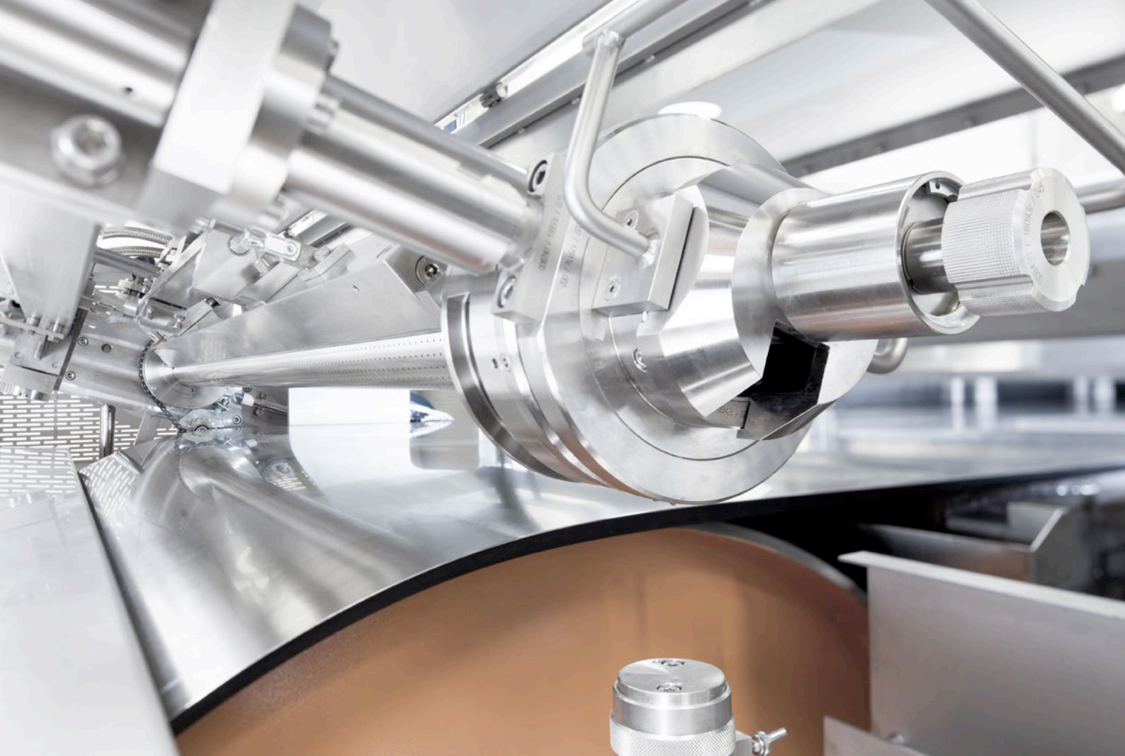
Premium solidification with Rotoform system. IPCO's Rotoform feed device.
